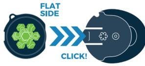
To clip in the snowcookie **PRESS** the release button downwards and slide the sensor flat side forward until clicks
